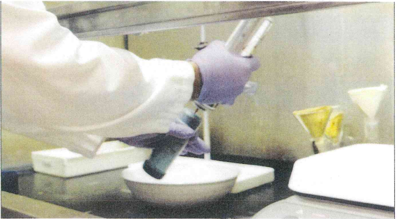
Top photograph: Marijuana placed in a plastic tube. The black cap has multiple holes with a paper filter inserted. The cap is then screwed on. Bottom photograph: Butane applied to the end of the tube of marijuana which travels through the marijuana, stripping the THC and depositing it in the white bowl.
