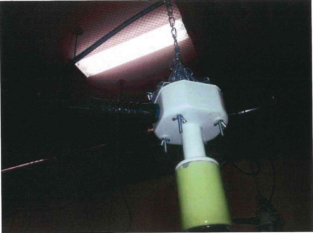
Lamp Assembly: Chained, 600V Lamp Cord w/ Strain Relief
